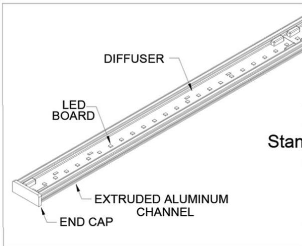
Standard pin-together lengths of 24", 12", 8" and 4".
