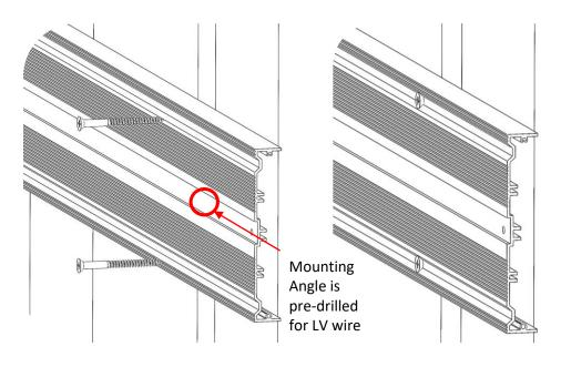
Attach the Mud-In bracket to the wall studs utilizing #8 self –tapping screws. Ensure the bracket is horizontal and level aligned with the wall surface; adjustments to the bracket are not possible once the drywall is cut and installed.
