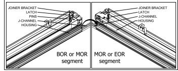
5. Note: case of WALL-to WALL installation. Remove reflector assembly from last but one segment. Remove joiner bracket screws. Slide joiner bracket and pins inside the housing. Install EOR segment as on Step 4. Slide joiner bracket back (bracket locator on housing edge). Secure joiner bracket with screws (see below left). Join run-thru harnesses inside housings with receptacle/plug connectors (see below right).
