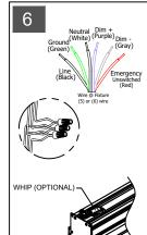
6. Make power/control wire connections as required in accordance with all applicable codes. Obey wire color codes (see on left). Replace reflector assembly. Use saved reflector mounting screws. Do not overtight screws, they could strip down aluminum housing. Connect whip as required if fixture supplied with whip. Make additional housing alignment if needed.
