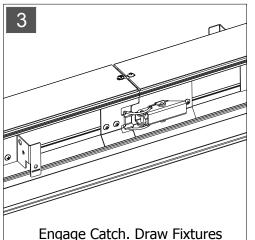
Engage Catch. Draw Fixtures Together and Close Latch.
