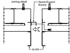
11. Install the Door Frames (use protective Gloves) by squeezing the torsion springs and inserted them into the torsion spring brackets in the Housing. Note: install spring with the lower tabs engaged and then repeat on the opposite side so door is suspended. Then carefully push the door upwards to engage into the housing assembly. Repeat as required.
