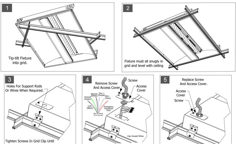
Screw Contacts Grid. Do Not Over-tighten.
