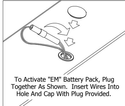
To Activate "EM" Battery Pack, Plug Together As Shown. Insert Wires Into Hole And Cap With Plug Provided.
