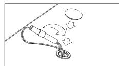
To activate "EM" battery pack, plug wires together as shown. Insert wires into hole and cap with plug provided.
