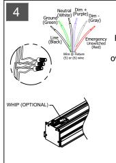
4. Make connections as required in accordance with all applicable codes. Obey wire color codes (see on left). Replace reflector assembly. Use saved reflector mounting screws. Do not overtight screws, they could strip down aluminum housing. Skip step 3 if fixture supplied with optional whip.
