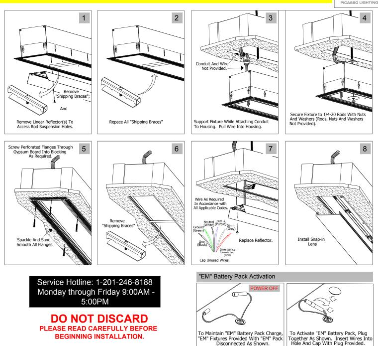
Installation and maintenance of the MAX4 luminaire may only be performed by qualified and licensed electricians in accordance with all applicable codes and standards.
