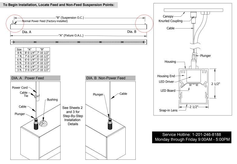
Position Canopy Over J-Box With Crossbar Stud And Wire Passing Through Hole In Canopy.
