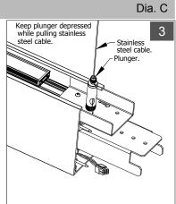
Trim cable. Allow length for adjustment if necessary.
